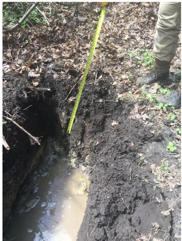
Photo 6. Excavated test pit in the upper reaches of the area of concern. Note the dark A p layer greater than 12 inches, with an underlying light-colored B horizon and standing water.
