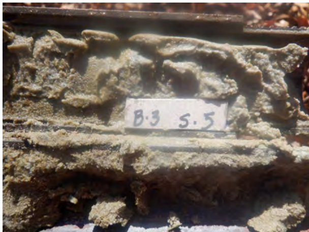
Photo 3: SP in B3 at 10 ft.; fine sand, wet
