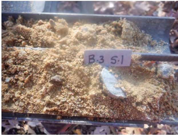
Photo 1: SP Glacial Fluvial in B3 at 1 ft; sand
