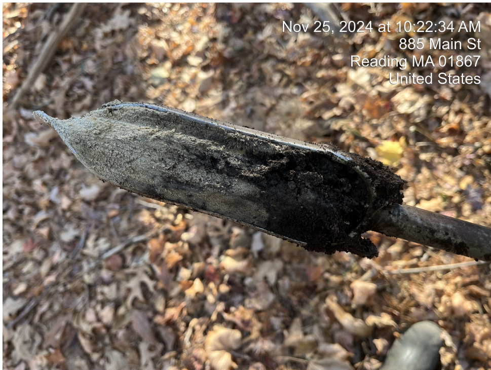
Photo 2: A view of a site typical depleted wetland subsoil, taken downgradient of GC A23
