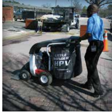
Figure 18. Walk-behind vacuum cleans a small parking area.
