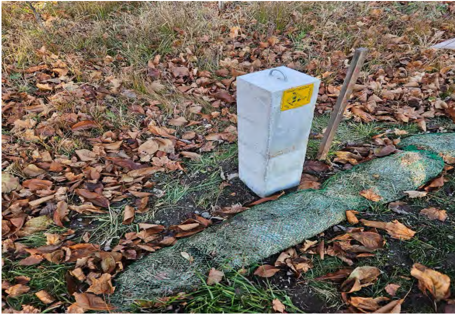
Photo #15: Photo of monumentation on edge of Zone of Natural Vegetation. Photo taken on November 28, 2023, by Hancock Associates staff scientist.
