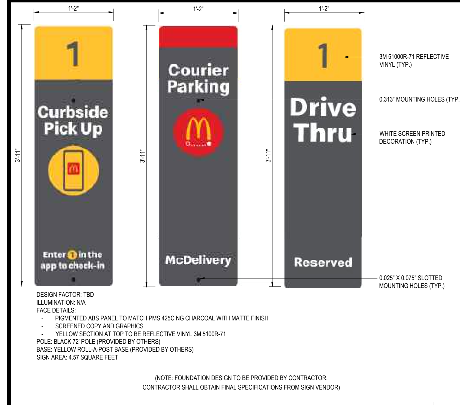
CURBSIDE PICKUP, McDELIVERY & DRIVE-THRU RESERVED SIGNS N.T.S.
